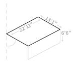
Shaded Area: Width up to 22' 11" Projection up to 13' 1" Pitch 10° up to 40° Drop Screen up to 6' 6"
