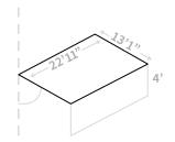
**Width** up to 22' 11" Projection up to 13' 1" Drop Screen up to 4'
